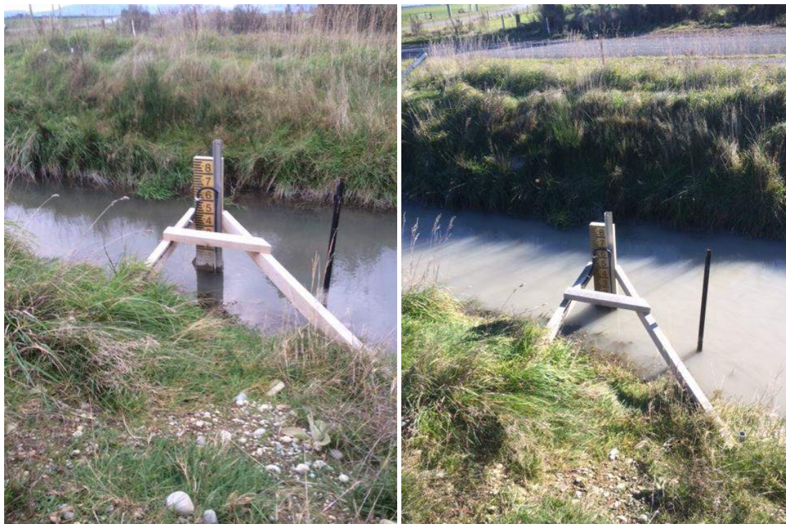
Figure I3: Valetta water race at Flume 2 with (a) normal and (b) high suspended sediment concentrations.
