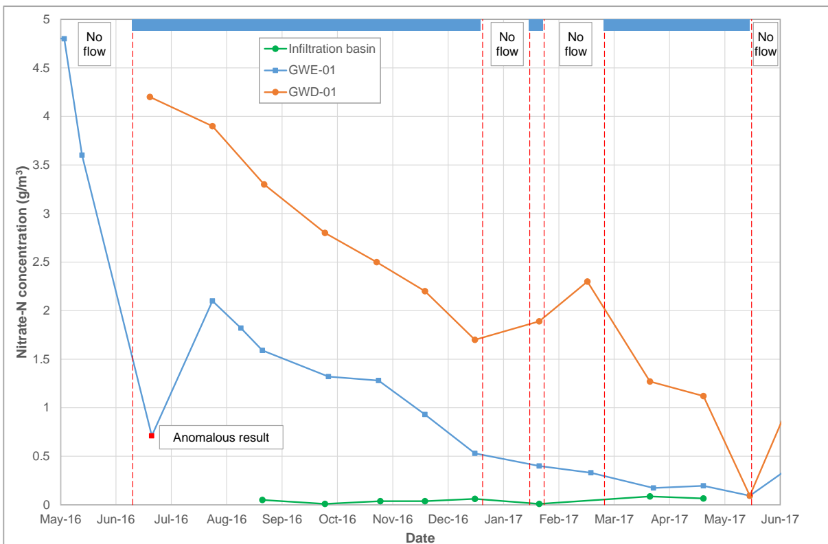
Figure H14: Nitrate-N concentrations in groundwater samples from beneath the Pilot Trial site during the trial.
