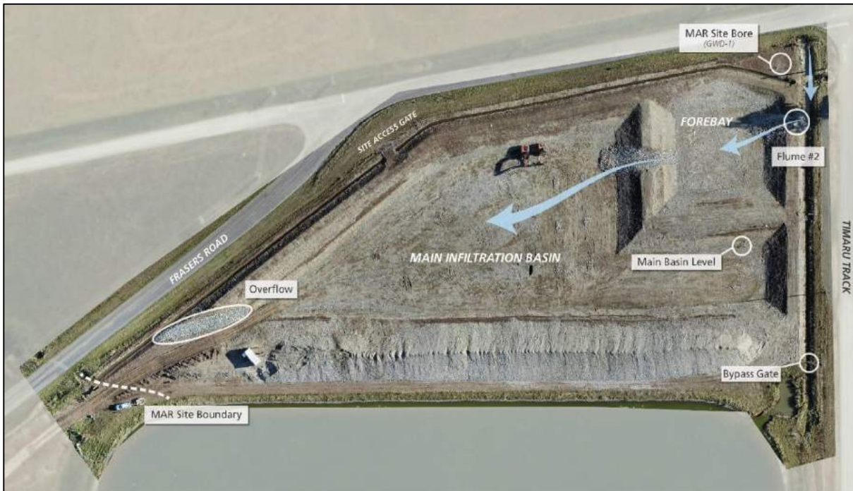
Figure E2: MAR Pilot Trial facility with key site structural and flow measurement locations.
