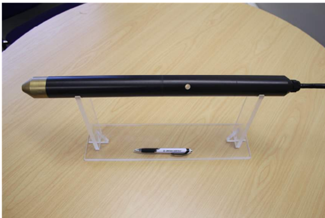
Figure 1: LAL prototype nitrate sensor showing black plastic body, brass 'sinker' and pass-through quartz sight glass
