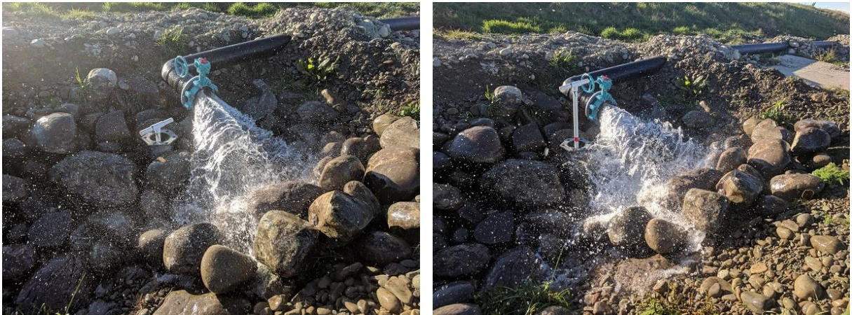
Figure 35: Red tag on floating level gauge indicates groundwater level compliance change (left in compliance and right outside compliance) following a change in pond water level.
